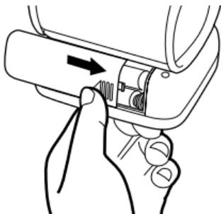
**REMOVING THE BATTERIES**
