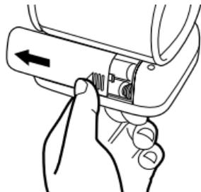
Pressing down on the battery cover, slide the cover off in the direction of the arrow.
